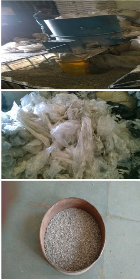
Fig. 1 Plastic shredding machine and shredded plastic
